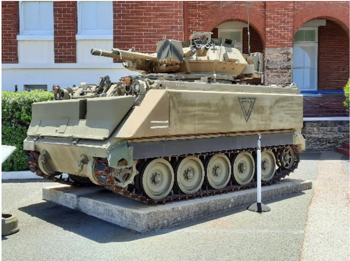
The Australian designed and built modification of the American M113 to accept the British Scorpion turret in the Fire Support vehicle.
