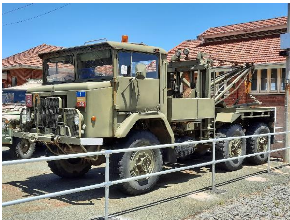
The Australian designed and built Light Wrecker using a Holmes recovery rig on an International Harvester chassis.
