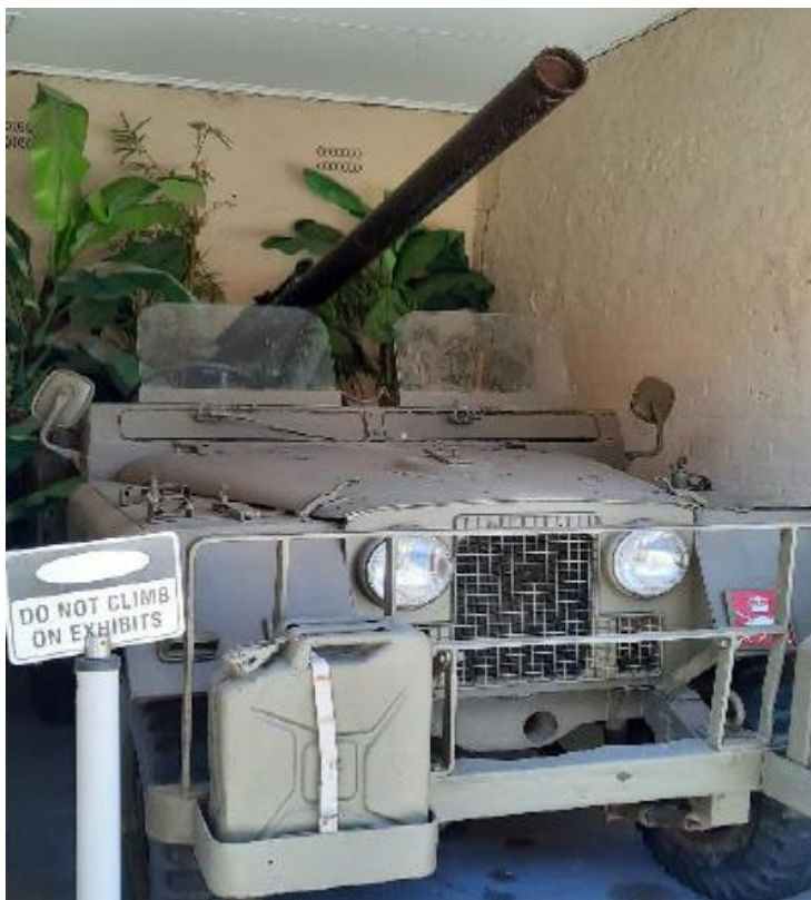
The Australian designed and built modification of the British Landover Series 2 to accept the American 106mm Recoilless rifle.
